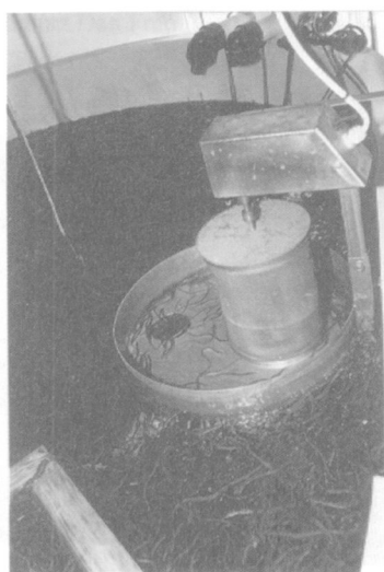
Fig. 1.12. Installation with brush to remove solids from the water (Kibbutz Dan Frame).
